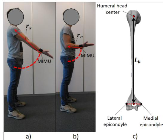
**Figure 1. Experimental setup. a) Shoulder elevation in the sagittal plane; b) elbow flexion-extension;**
