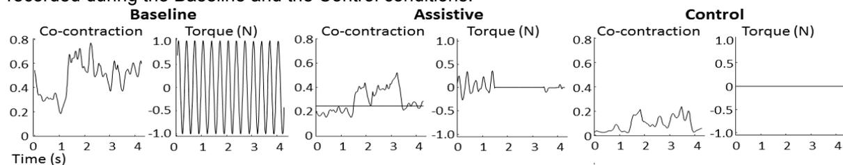
**Figure 1.** Examples of the level of co-contraction and torque perturbations. The line reported in the Assistive condition represents the boundary of 0.25 above which no torque were exerted.
