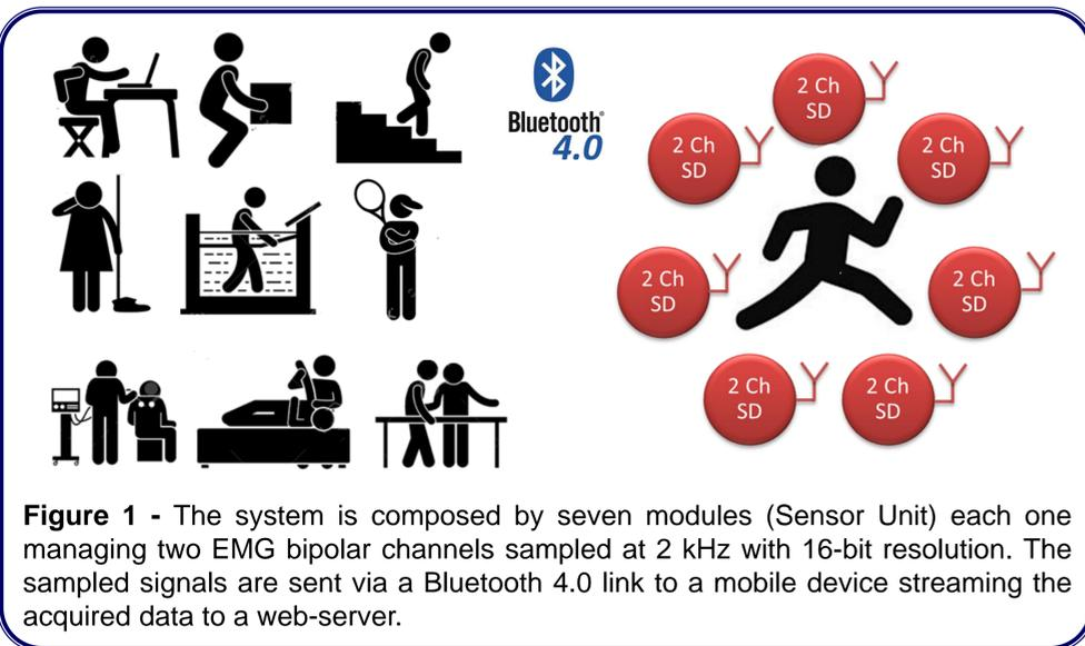
**Figure 1** - The system is composed by seven modules (Sensor Unit) each one managing two EMG bipolar channels sampled at 2 kHz with 16-bit resolution. The sampled signals are sent via a Bluetooth 4.0 link to a mobile device streaming the acquired data to a web-server.
