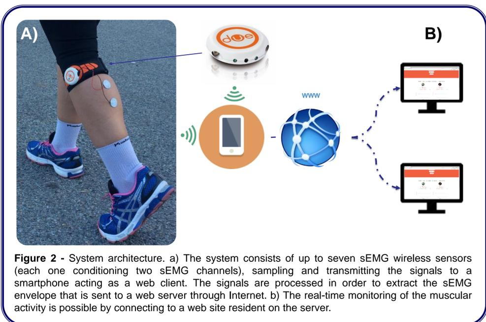
**Figure 2** - System architecture. a) The system consists of up to seven sEMG wireless sensors (each one conditioning two sEMG channels), sampling and transmitting the signals to a smartphone acting as a web client. The signals are processed in order to extract the sEMG envelope that is sent to a web server through Internet. b) The real-time monitoring of the muscular activity is possible by connecting to a web site resident on the server.
